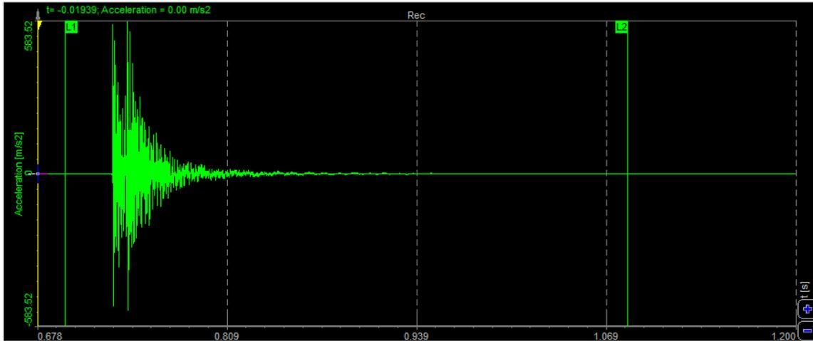
The channel cursor (yellow cursor) that indicates our position in the timeline of the datafile has to be placed at the beginning of the shock.
