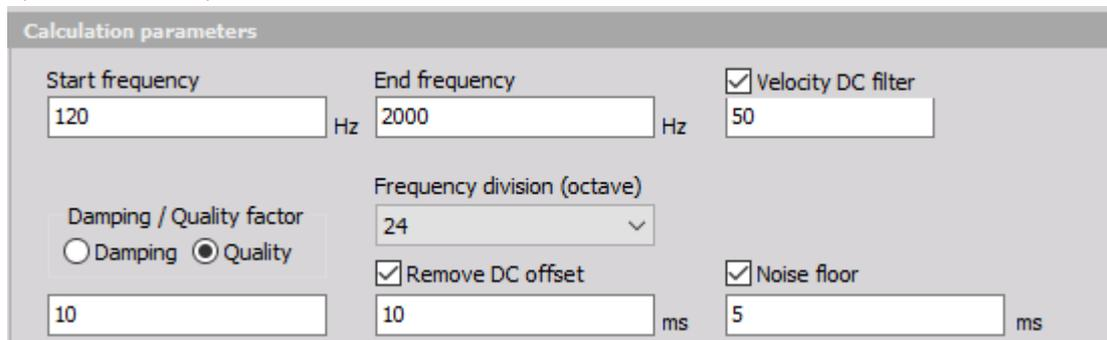
**Start** and **end frequency** define the calculation range for the frequency spectrum. The upper limit is set to 1/2 of MAX sampling rate.
