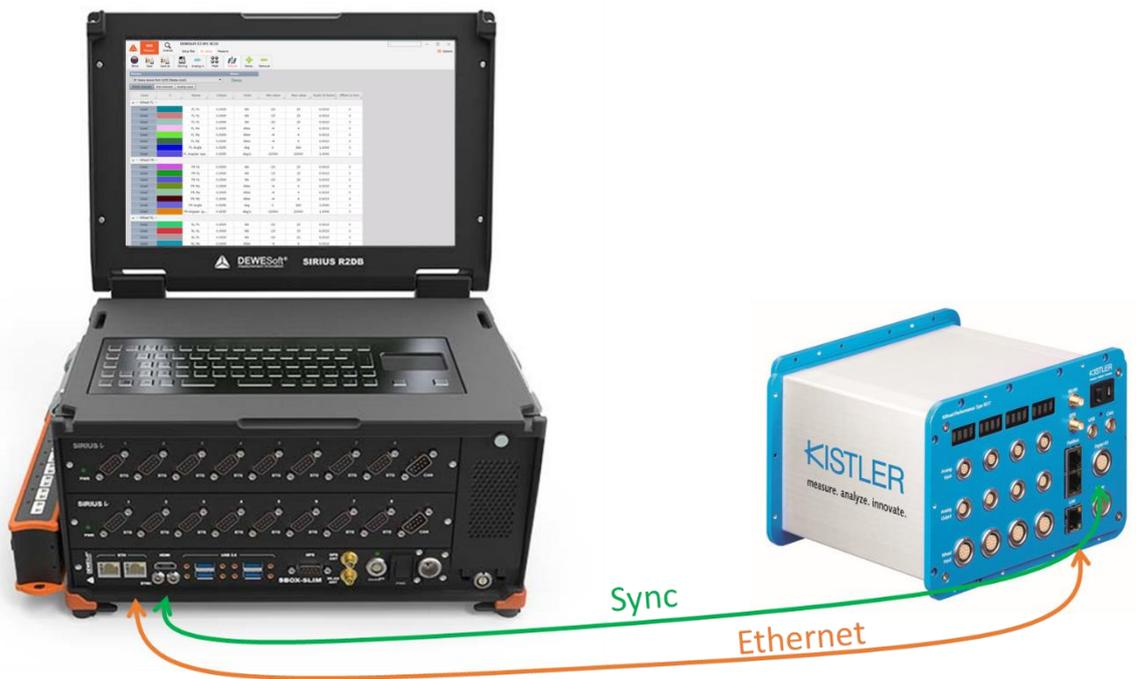
Figure 7 - Hardware connection
