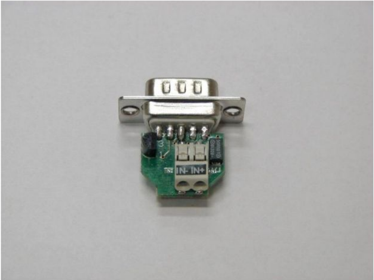
Illustration 6: MSI 20mA top assembly
