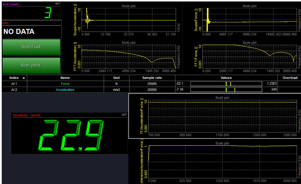
Sensitivity of our hammer is 22.9 mV/N. We use this information in Setup at Channel 1.
