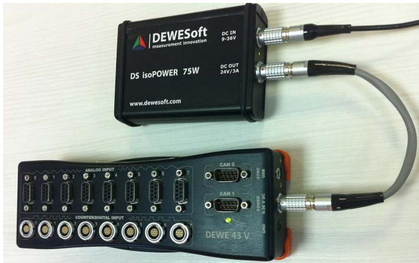
The final result is the same: reverse polarity protection of the supply line.
