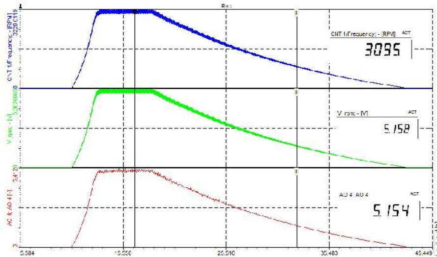
The max measured RPM is 3095, which equals 5,15V.
