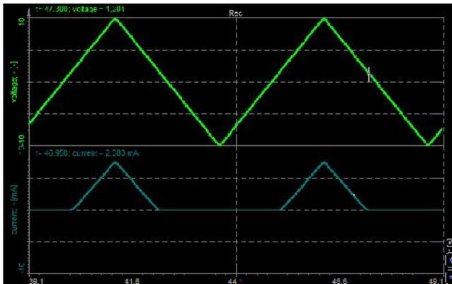
Use a XY recorder, assign “voltage” to the x- and “current” to the y- axis to get the characteristic line of the diode and measure the forward voltage, in this case about 1,65 V.
