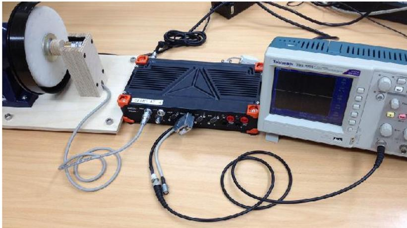
The Encoder on the left side is mounted on a grinder bench. It is connected to the ACC+ counter input on channel 1. On the MULTI module on channel 4 a special split-adapter is connected, the analog output is routed to the oscilloscope.
