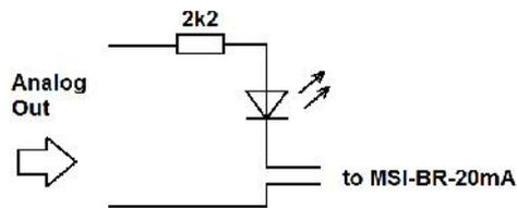
In this simple circuit the AO is connected to a LED over a resistor with 2k2 ohms (to limit the current), to the MSI-BR-20mA for current measurement.
