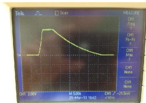
Also on the scope you see the correct max RPM (approx. 5,2 V).
