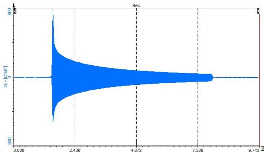
In this example the max amplitude is approx. 600 um/m.
