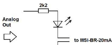
Enable the Analog channel you want to use and select a triangular waveform with an amplitude of 10V peak (signal will go +/- 10 V):
