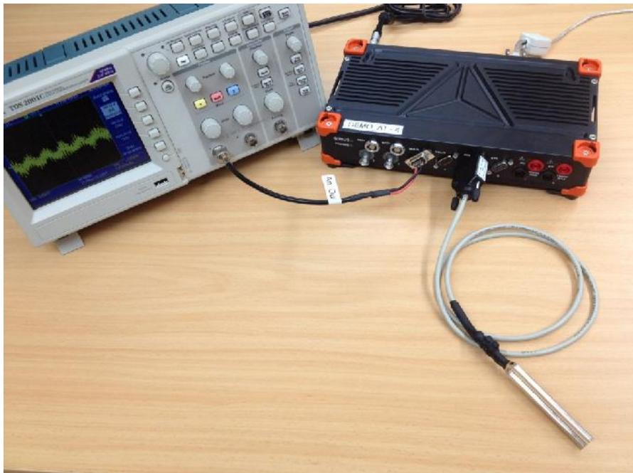
We use a strain gage with strain scaling (um/m). Do one hit, store a datafile:
